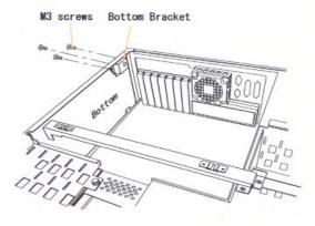
Remove the HDD expansion unit from the 2200 Plus Removable Tray. Install HDD (two HDD can be installed) into the unit and put it back to the former position.
