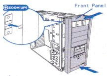
ere are USB cable, Power SW, Reset SW, d LED cable attached to the back of the ont Panel. Do not damage those cables ien installing the Front Panel. There are so some secure pins on the back of the ont Panel. When installing the Front nel to the main case, those pins should be serted into the matching holes of the case.
