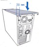
VII. Fasten with the two screws on the back of the cover.
