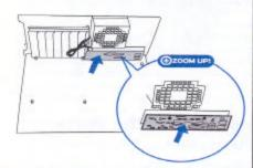
IV. Use M3 screws to fasten the Motherboard. Do not touch the printed wires on the motherboard when fastening with the
