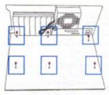
ii. In the event of replacing ATX I/O Shield Bracket according to your motherboard ATX I/O layout, remove the bracket by pushing into the case.
