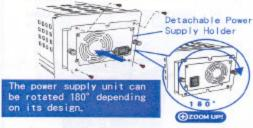
Some Power Supply Units cannot be installed depending on the design.
