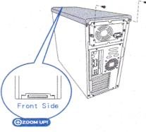
There is a securing tab on the back of the top cover. Use the tab to hold the chassis firmly.
